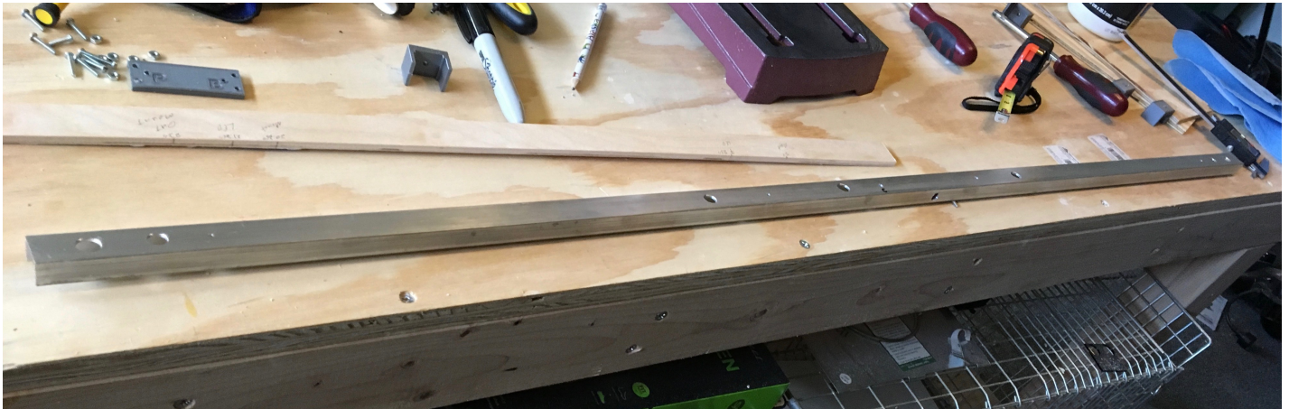
Figure 13: Channel completely drilled. Note 5/16 hole on side of Channel for power jack
