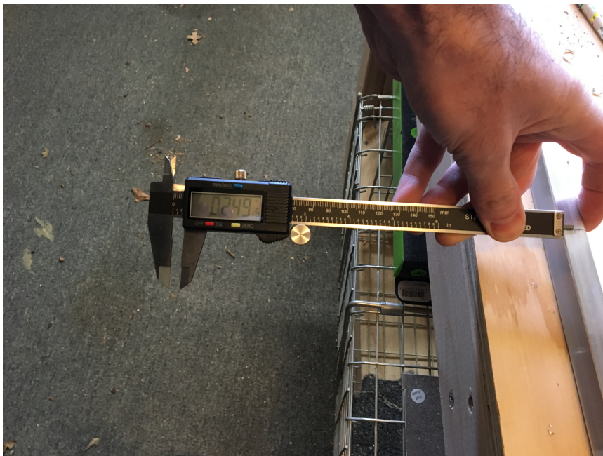
Figure 12: Make mark 1/4" away from the open edge of channel, roughly 2.5" down from button hole. Drill a 1/8" pilot hole followed by a 5/16" hole for power jack entry
